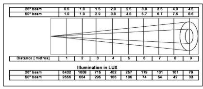
For best results the unit is shipped with the GE Precise 50W 25° 12V MR16 lamp.. **Note**: The BeamShaper uses Selecon's custom designed aspheric lens to minimise beam distortion and field curvature resulting in excellent pattern projection for a luminaire of this type. The actual performance is dictated by the lamp used.
