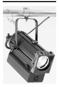
High intensity display luminaire with adjustable 7°– 60° soft edge beam for controlled illumination using the popular long life 250W 6700°K MSD lamp. The adjustable spot to medium flood beam is easily blended with adjacent beams and can be shaped using the 4-door barndoor accessory.
